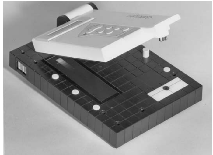
Darklight Duo Combination Sensitometer and Densitometer with Automatic Scanning
